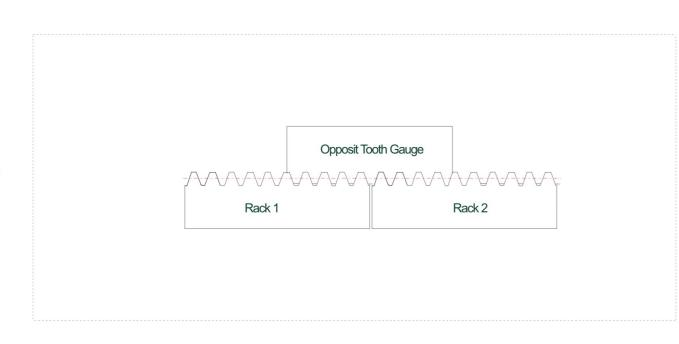
The figure above shows how to use the Opposit teeth gauge to connect two racks to a standard pitch. To check the Opposit tooth gauge accuracy, use the gauge shown in the figure below to measure.
