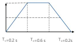
With same pulley diameter you want to obtain a displacement of 1 meter in one second.
