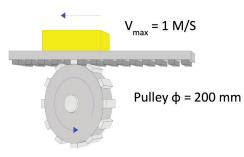
You simply need to divide the speed by the pulley radius in meter = 0.1 m It gives you the rotational speed of the pulley in radians /second = 1 / 0.1 = 10 rd/s If you divide by  $2\pi$  and multiply by 60 you obtain rotational speed in rpm
