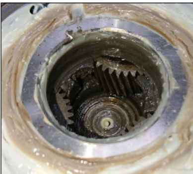
The internal wear of gear reducers. Shown here: Input 3,000 rpm, 100 hours, total of 18 million revolutions.
